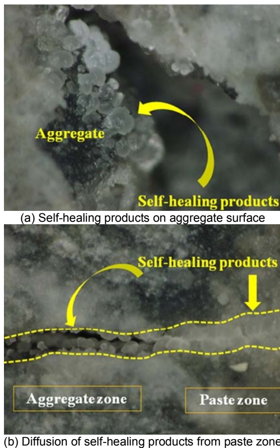
Fig. 27 Self-healing images on crack between aggregate zone and paste zone of self-healing concrete.
