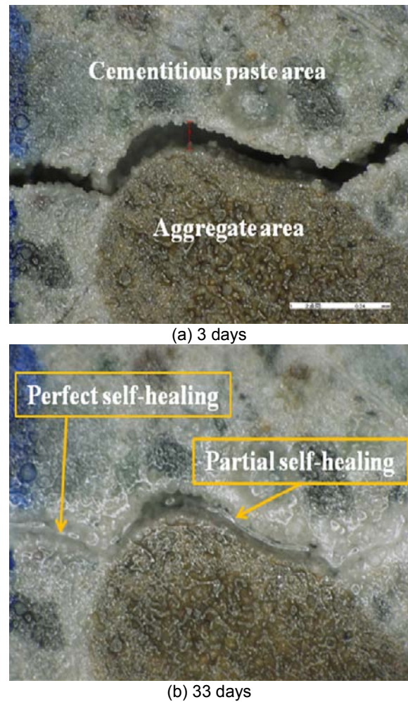
Fig. 26 Process of self-healing on self-healing concrete at water/binder ratio of 0.47.
