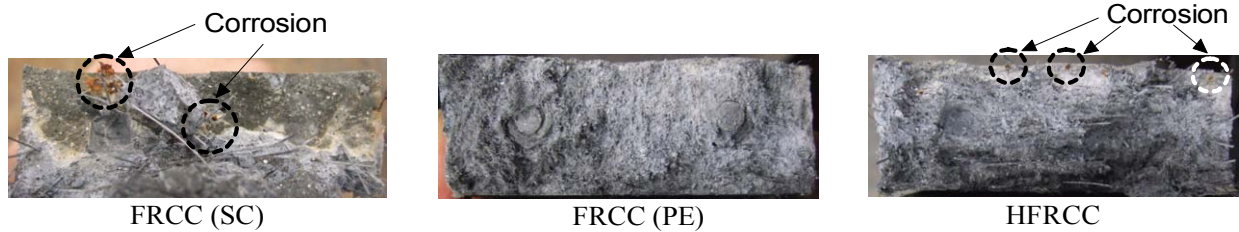
Fig. 16 Comparison of crack surface after second tension test.
